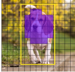
Figure 17 Multiple Grids may detect the same object NMS is used to remove multiple detections
