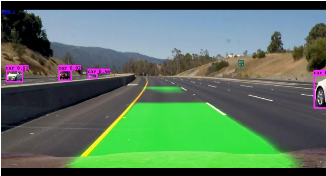
Figure 18 Detecting objects and the lane Simulation.
