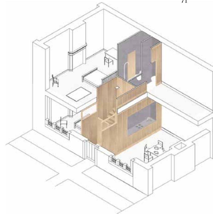
[5] Memory as a design studio: the large oak furniture-objects restructuring the vertical rhythm of the houses, including staircases and other services. This is inspired by the original cabinets of the beguines, which offered them some privacy.
