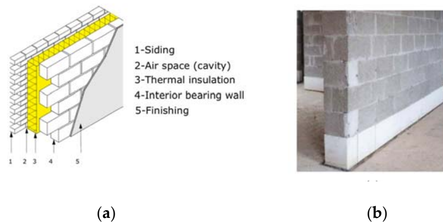
Figure 1. (a) Cavity wall, adapted from WTCB (2016) [5]; (b) masonry wall composed with a thermal break layer at the bottom, reprinted from XELLA (2016) [6].
