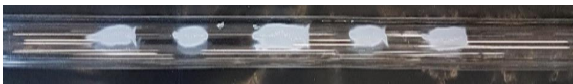
Figure A2. Erosion on the inside of a 4.8 mm (ID) × 7 mm (OD) glass tube after being exposed to the highest amplitude for 2–4 h. The white zones show erosion of glass. Smaller tubes (4 mm OD) hardly showed any erosion.
