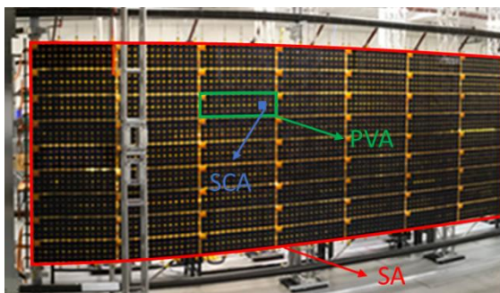
Figure 1: Example of a rollable SA (ROSA) [3]
