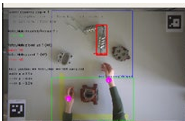
Fig. 5. The state tracker monitors the process. Red area: Part to be picked detection. Pink dots: operator's hands detection
