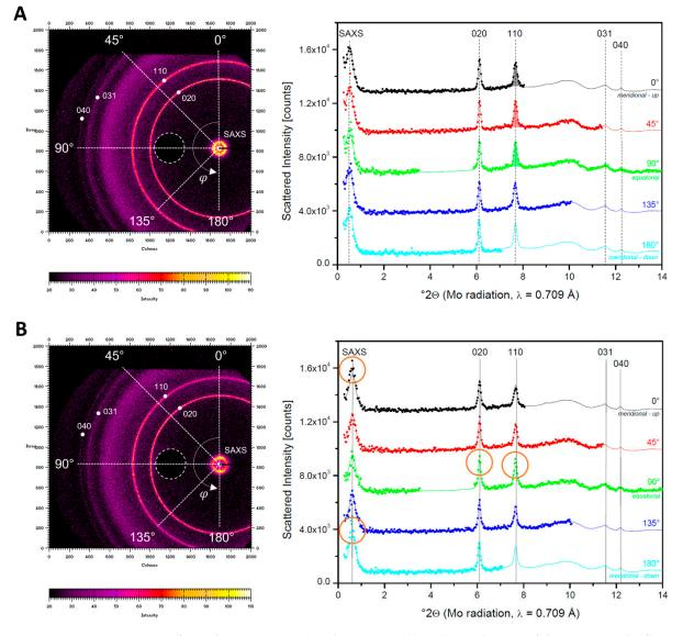
**Figure 9.** 2D scattering patterns of samples  $\mathbf{M} = 80 \,^{\circ}\text{C}$  (**A**) and  $\mathbf{M} = 40 \,^{\circ}\text{C}$  (**B**) with an indication of the PHB typical reflections with Miller indices (**left**) and corresponding individual scans along different  $\varphi$  directions (**right**). The white circled regions in the 2D scattering patterns are detector blind regions.
