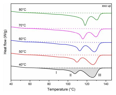
**Figure 6.** DSC first heating curves of PHBHHx samples with variable mold temperatures  $\mathbf{M} = 40$  to 80 °C with three endothermal peaks (I–III) for crystallinity calculations.
