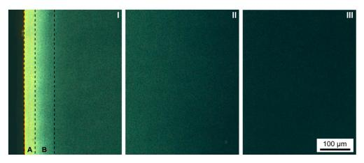
**Figure 7.** Optical analysis. POM micrographs on 40  $\mu$ m thin sections with mold temperature **M** = 40 °C showing birefringence gradient existing in the different regions from the skin to the core (**I–III**). (**A**) and (**B**) represent the skin and shear-like layers, respectively.
