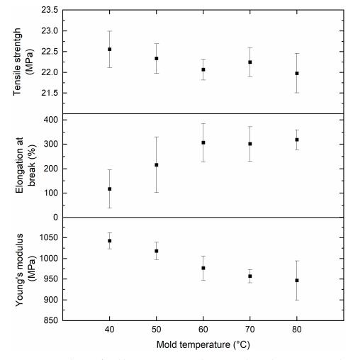
molded PHBHHx, other differences in microstructure, orientation effects, in particular, are investigated hereafter to account for the observed variations in mechanical properties.
