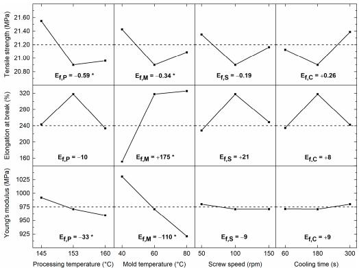
**Figure 3.** Main effects plot for tensile strength (TS), elongation at break ( $\varepsilon$ ), and Young's modulus (E) showing average values across the FFD matrix for the parameters **M**, **P**, **S**, and **C**. Significant main effects E<sub>f,X</sub> are indicated with an asterisk.
