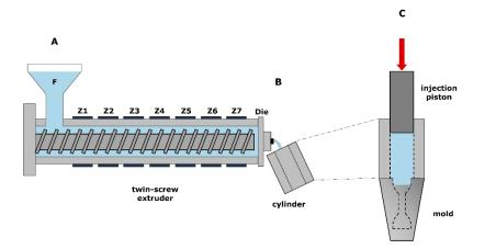
**Figure 1.** Three-step PHA melt processing with twin-screw extrusion through nine temperature zones (**A**), melt transfer into heated injection cylinder (**B**) and piston melt injection into a heated dumbbell-shaped mold (**C**).
