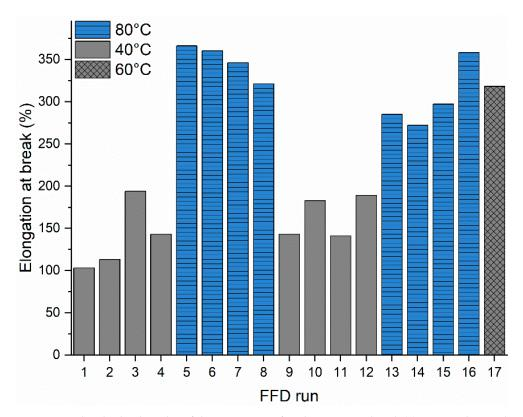
**Figure 4.** Individual value plot of the 17 run FFD for elongation at break ( $\varepsilon$ ), grouped according to mold temperature **M** = 40 °C (grey), **M** = 80 °C (blue), and **M** = 60 °C center point run (grey, cross) showing increased elongation at break for high mold temperatures (only mean values are represented for clarity, statistical error is included in Table 4).
