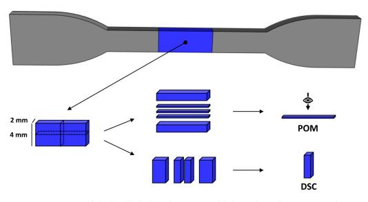
**Figure 2.** Dimensions of the dumbbell-shaped injection molded samples and cross-sections for POM and DSC analysis.
