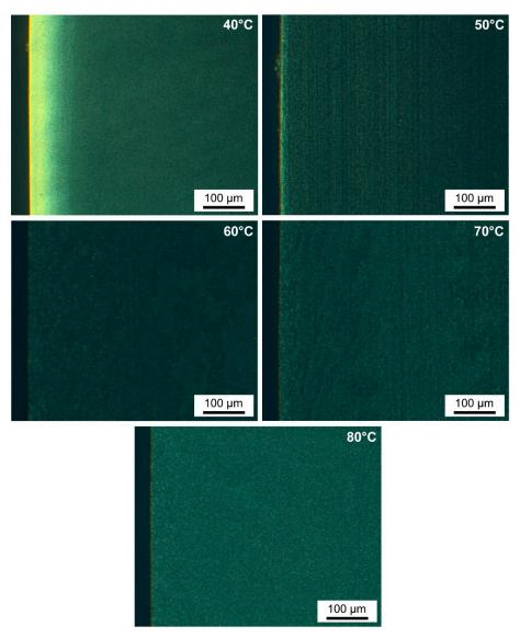
Figure 8. POM micrographs with 20  $\times$  zoom on 40  $\mu m$  thin sections for mold temperatures M ranging from 40–80 °C.
