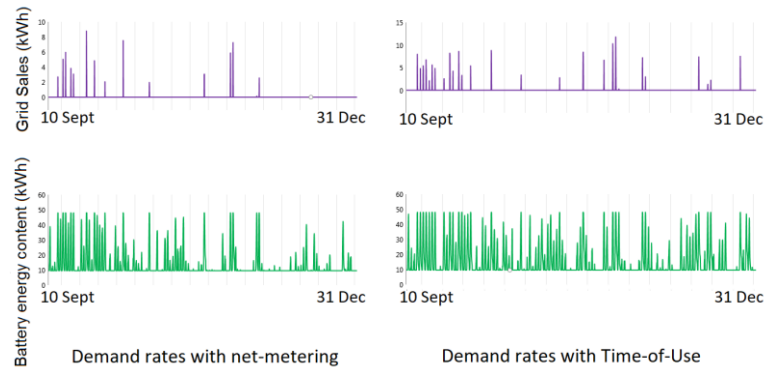
Figure 2. Energy sales to the main grid (kWh) and Battery energy content (kWh) for the microgrid system for the last quarter of a year in Spain, with Demand Rates added to the volumetric pricing schemes
