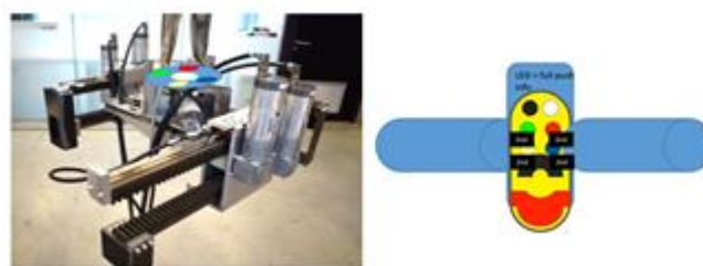
Figure 8: Rough sketch of the (envisioned) led notifications for showing system status and the gripper handle with room for the magnetic controller in the middle
