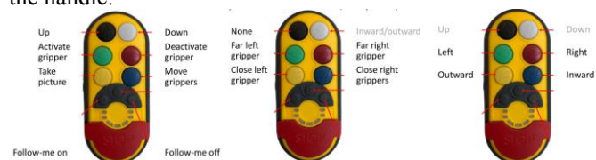
Figure 7: Wireless controller with default button assignment, axis selection for manual movement and actions when a horizontal axis is selected
