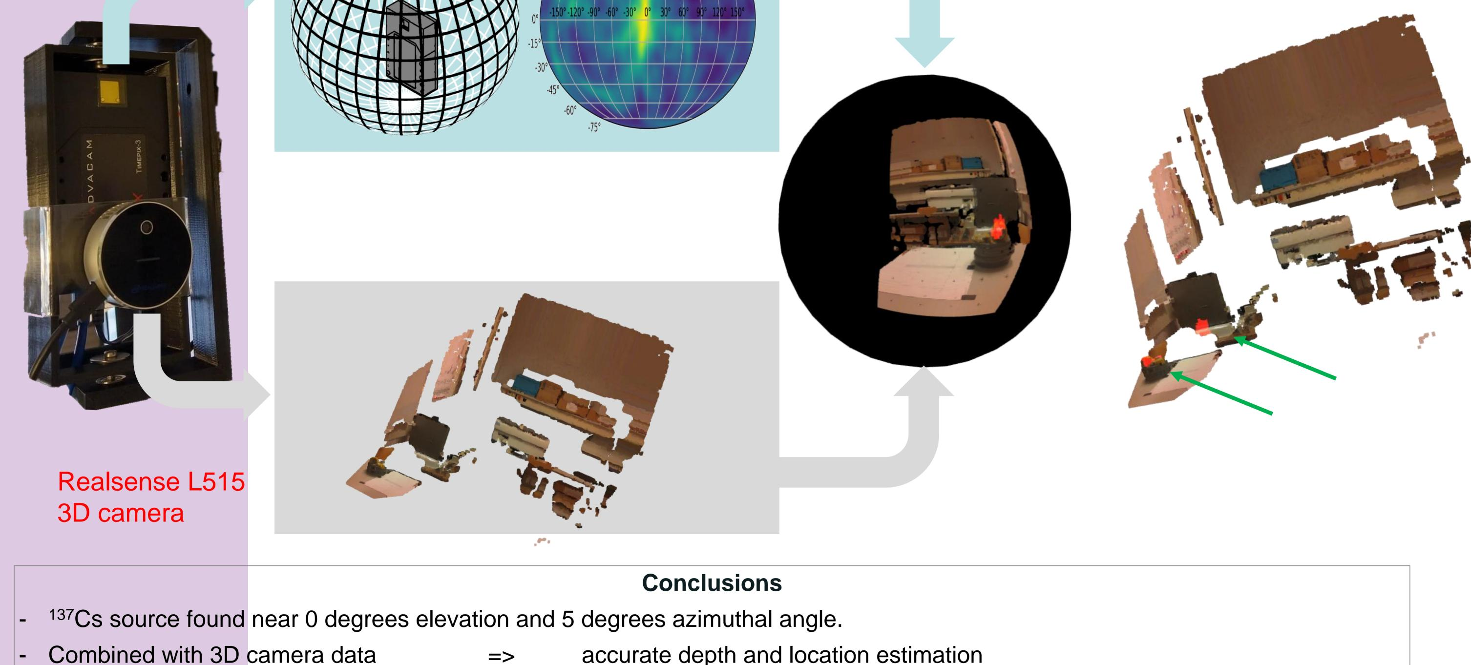
False hotspot found behind real source => eliminate with second measurement from side
