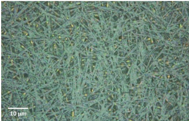
Fig. 2. Fiber-like structures observed by optical microscopy after the ultrasonic spray coating of perovskite with slow solvent evaporation.
