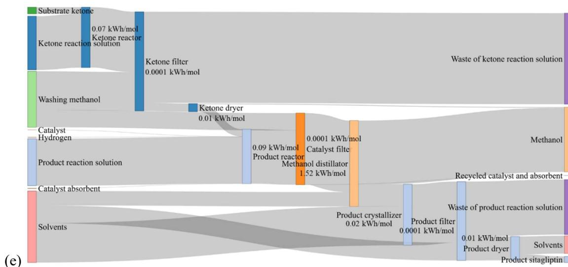
**Figure 5.** Mass flow and energy consumption (a) Case 1 for MBA production; (b) Case 2 for MBA production; (c) Case 1 for sitagliptin production; (d) Case 3 for sitagliptin production; (e) Case 4 for sitagliptin production.
