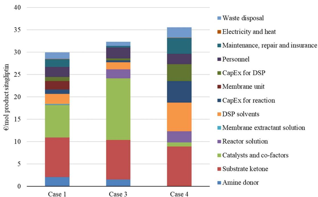
**Figure 7.** Breakdown of process and downstream costs (CapEx and OpEx) to produce sitagliptin for Cases 1, 3, and 4.
