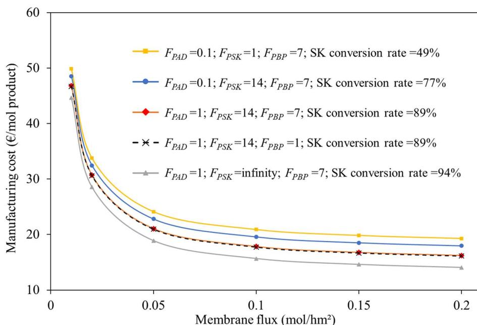
**Figure 12.** Manufacturing costs of Case 1 as functions of membrane flux of product amine, the concentration ratios of product amine/amine donor ( $F_{PAD}$ ), product amine/substrate ketone ( $F_{PSK}$ ) and product amine/by-product ketone ( $F_{PBP}$ ) in the extractant solution; substrate ketone (SK).
