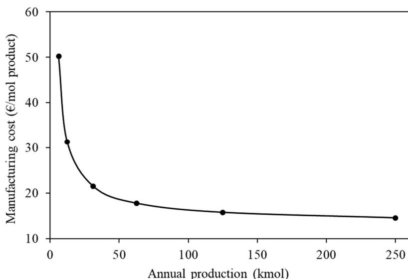
**Figure 9.** The manufacturing cost of Case 1 as a function of the annual production.
