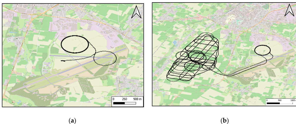
Figure 12. (a) Flight path of the first flight with the circular pattern. (b) Flight path of the second flight with the circular pattern and the grid pattern.
