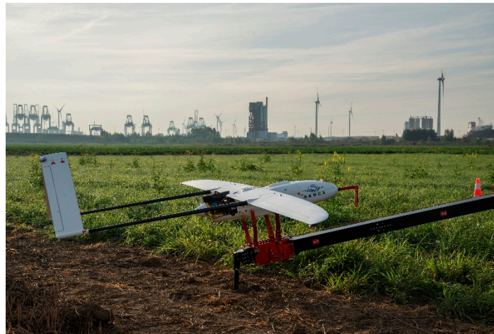
Figure 1. Penguin C UAV from SABCA mounted on the pressurized catapult.
