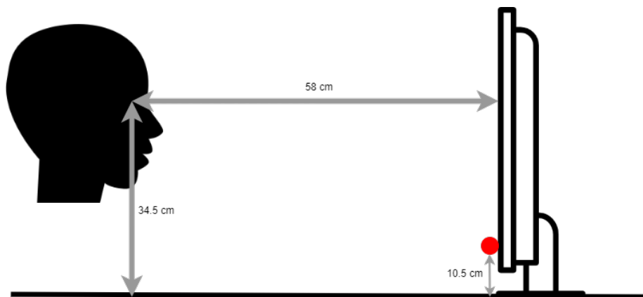
Figure 3.6: Position of test subject during the gaze calibration test.
