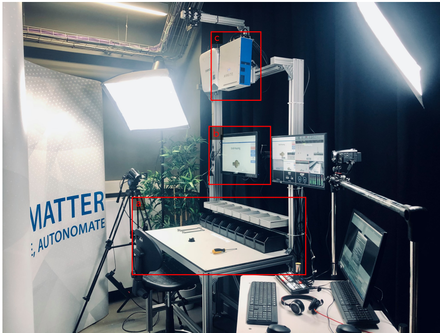
Figure 1.1: Example of a possible Human Interface Mate (HIM) setup. a) Working station where projection of the HIM will be projected to, b) monitor where instruction set will be shown, c) the HIM.
