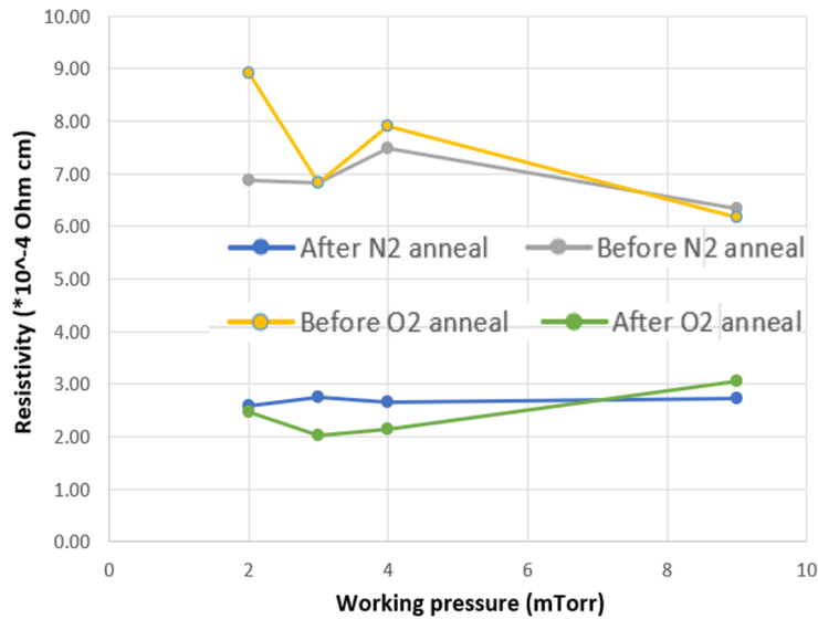
Figure 4.18: Resistivity of ITO before and after either O 2 or N 2 anneal at 200°C
