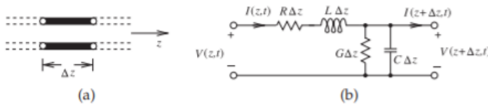
Transmission line segment: (a) of length \Delta z ; and (b) lumped-element model.
