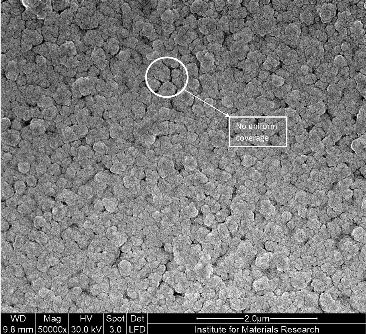
Figure 53: SEM picture of 80 layers with pinholes.
