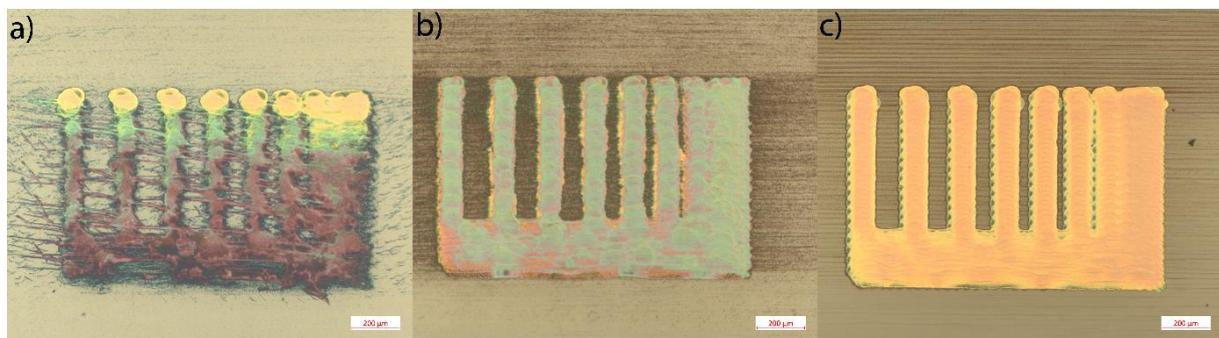
Figure 89: comparison of inkjetted patterns.  $O_2$ -plasma treatment after four days (a),  $O_2$ -plasma treatment after six days (b),  $O_2$ -plasma treatment after 16 days (c).
