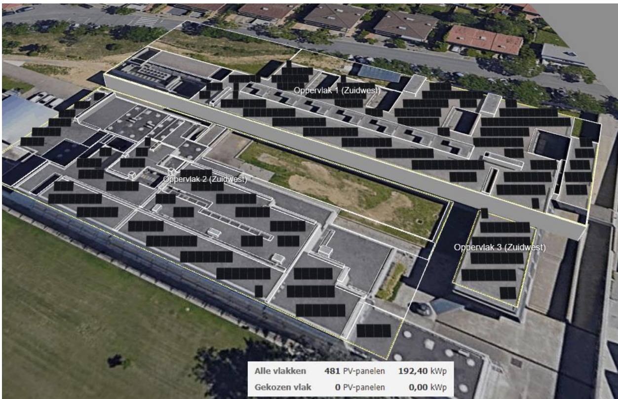
Figure 58: Configuration P1 building_ SPR-MAX3-400
