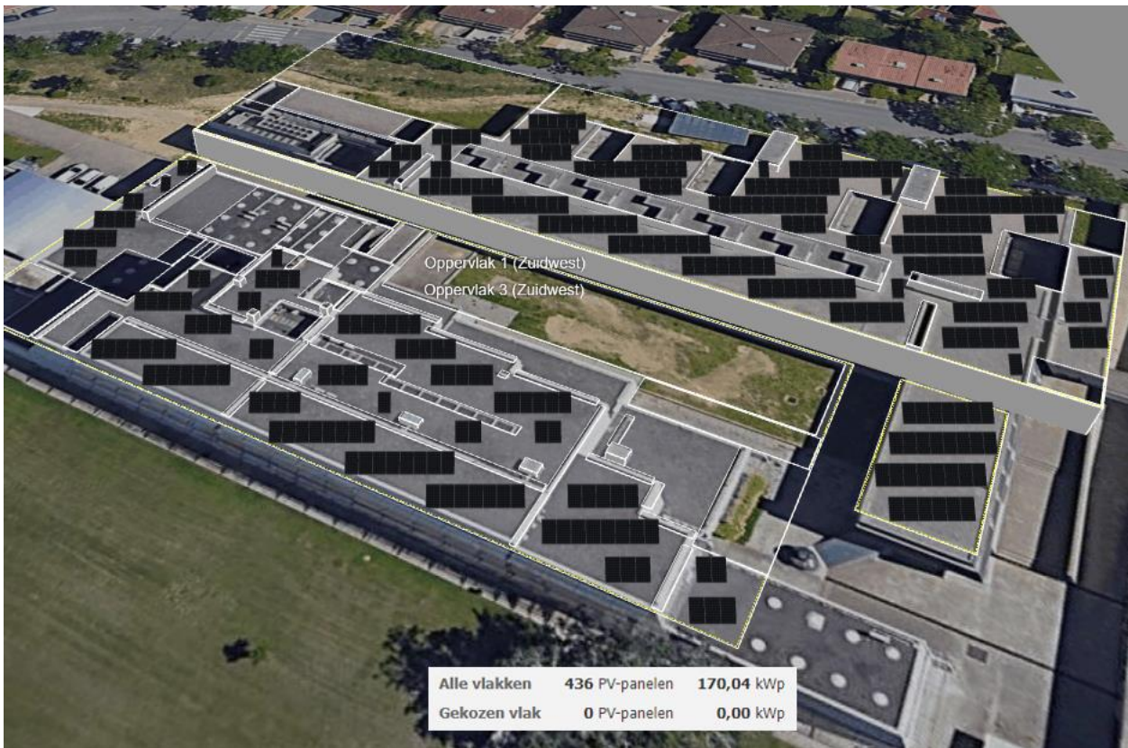
Figure 59: Configuration P1 building_ JKM390M-6RL3-B
