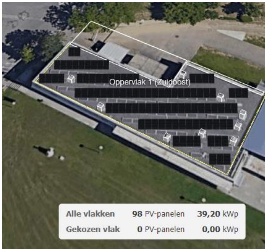
Figure 79: Configuration P3 building_ SPR-MAX3-400
