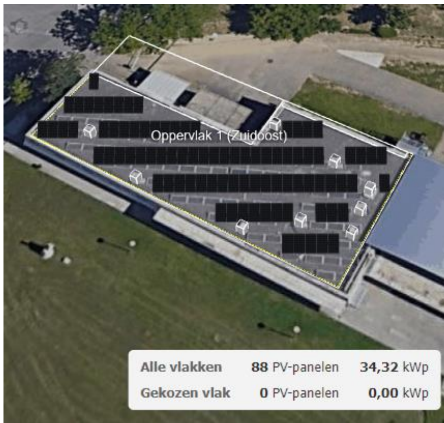
Figure 80: Configuration P3 building_ JKM390M-6RL3-B
