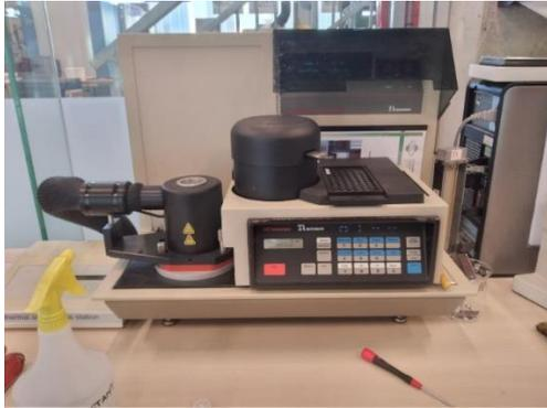
Figure 24: DSC Autosampler (TA Instruments).
