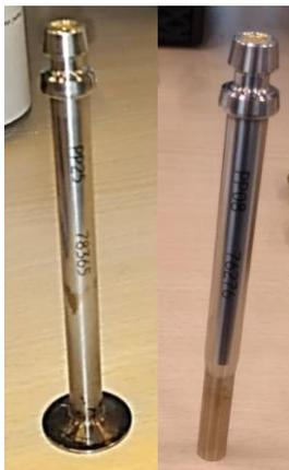
Figure 23: PP25 (79044) parallel plate probe (left) and PP08 (5681) (right).
