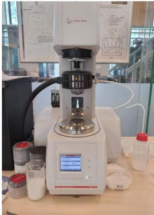
Figure 22: MCR302e Rotational Compact Disk rheometer (Anton Paar).
