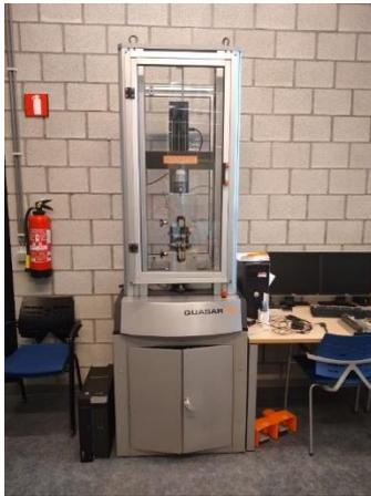
Figure 25: Quasar 50 kN tensile testing machine.
