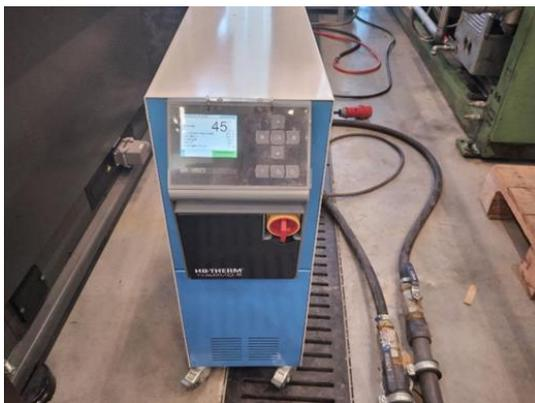
Figure 21: Thermo-5 (HB-180Z2) cooling unit (HB-THERM).
