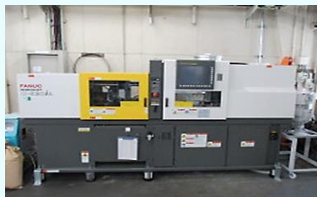
Figure 1: Fanuc ROBOSHOT S-2000i30B injection molding machine [3].
