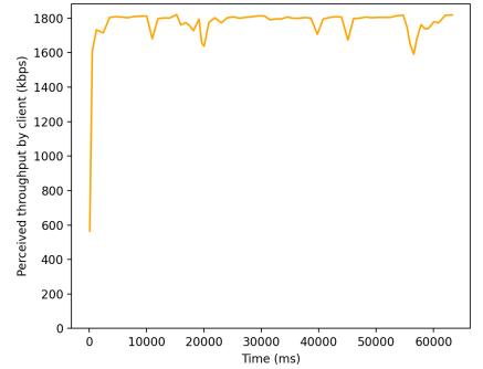
Throughput experienced by AverageXL during network simulation with throughput of 2mbps
