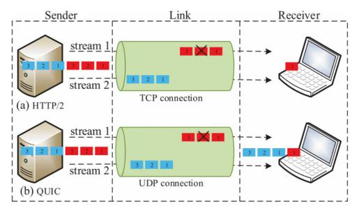
**Figure 2.5:** Visualisation of head-of-line blocking by Yu, Xu, and Yang 2017. a) shows multiplexing with HTTP/2 b) shows multiplexing with QUIC.
