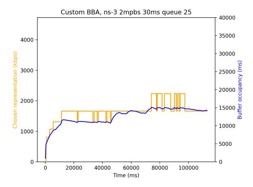
(a) Test using a constant throughput of 2mbps, a constant delay of 30ms and a packet queue of 25 in ns-3.
