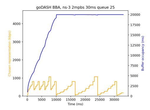
**Figure 4.10:** Selected bitrate and buffer occupancy of the BBA-2 implementation by goDASH with a video buffer size of 20 seconds. The chosen representation is displayed using the downloaded segments bitrate in kbps on the left y-axis. The buffer occupancy (buffer level), is displayed on the right y-axis in milliseconds. We would expect to see the chosen representation follow the line of the buffer occupancy if BBA was working as it should be.
