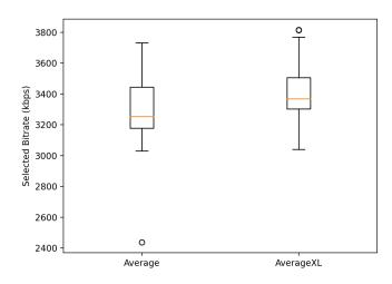
(a) Boxplots of the chosen bitrates by Average and AverageXL. The bitrate is shown in kbps and it defines the bitrate of the segments the algorithm chose to download.
