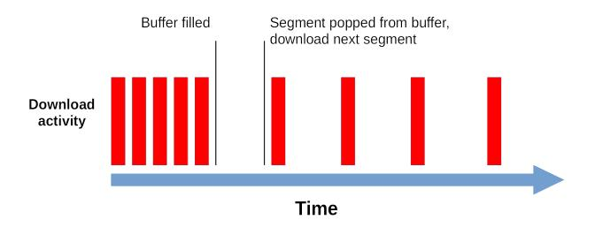
Figure 4.1: Visualisation of the on and off periods of network activity from an ABR client. During every red block, a segment is being downloaded. Between the segments is some idle time, because the ABR algorithm needs a little time to perform calculations. When the video buffer is filled, the next segment will only be downloaded when an entire segment is taken out of the video buffer for playback. At this point in the video stream, the periods of silence between the segments will be larger.
