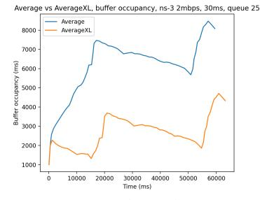
(a) Comparison of the buffer occupancy of Average and AverageXL with an ns-3 simulation.
