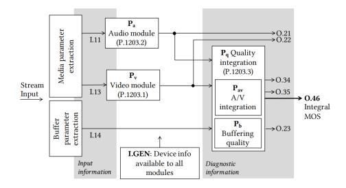
Figure 2.4: Input and output structure of P.1203, by Robitza et al. 2018.
