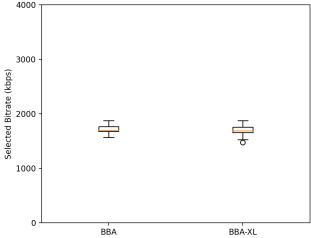
Selected bitrate of 20 tests with BBA and 20 tests with BBA-XL
