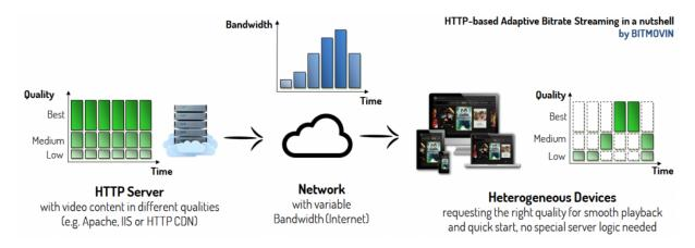
Figure 2.1: Structure of DASH streaming by Mueller 2019.
