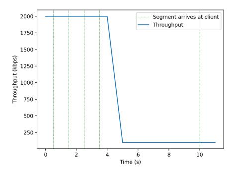
Figure 4.12: Hypothetical scenario that might cause BBA to experience stalling. The blue line shows the throughput the client would experience on the network over time. The vertical green lines indicate every point in time when a new segment arrives at the client. After the fourth green line, the fifth segment has just started downloading. When the throughput suddenly drops, that same segment will take a lot longer to arrive at the client.
