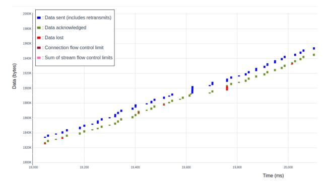
Figure 4.5: Congestion graph showing the smaller gaps between segments when the ITU P.1203 script is not executed for the Average algorithm of goDASH. The congestion graph shows how much data is in flight (blue) at what point in time, and when they are acknowledged by the receiver (blue). The gap is only about 60ms now, which is a lot better than the 200ms we had previously.
