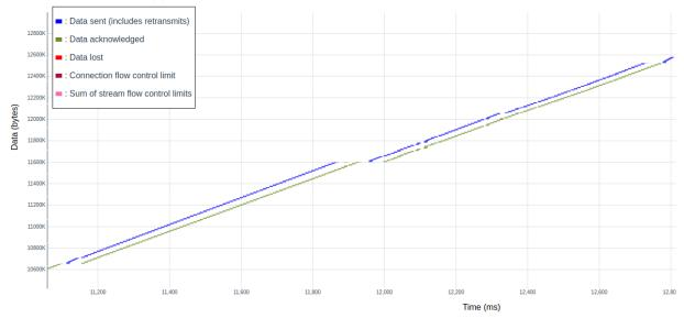
(b) Enlarged graph showing the large gap between two segments. The gap that dash.js has between its segments is a lot shorter than what we see with Average of goDASH in Figure 4.3.
