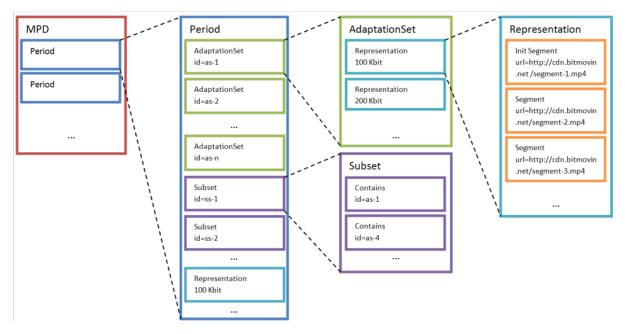
Figure 2.2: Structure of a DASH MPD file by Mueller 2019.
