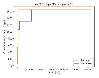
(b) Comparison of the chosen representation between Average and AverageXL with an ns-3 simulation. The representation is the quality level of segments the algorithms choose to download. They are displayed in kbps, according to the bitrate of the chosen segment. AverageXL (in orange) chose a representation with a bitrate of 1600kbps earlier than Average (in blue).
