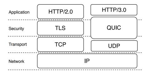
Figure 2.6: Protocol stack of a secure HTTP/2 connection compared to HTTP/3, by Mehdi Yosofie 2019.
