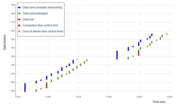
(b) Enlarged graph showing the large gap between two segments. This is about 200ms. This is a lot longer than it should take for an ABR algorithm to do the calculations and start downloading the next segment.
