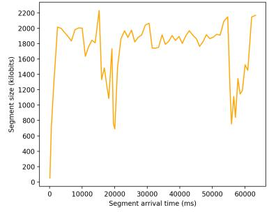
Figure 4.8: This is the size of the segments that AverageXL downloaded during the ns-3 test from Figure 4.6. The fluctuation shows the difference between the sizes of segments from the same representation.
