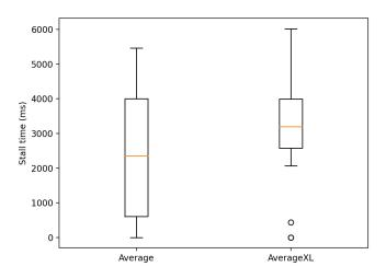
(c) Boxplots of the total amounts of stalling the clients experienced using Average and AverageXL. Fewer seconds spent stalling is desirable.
