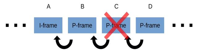
Figure 3.1: Example of losing a P-frame during a video stream. P-frames base pixel information on the previous frame.
