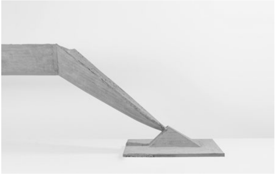
Fig. 7.12 Folded beam of a roof structure, model in concrete. Cultural Centre Lokeren, competition design, not executed, Architect Juliaan Lampens, approx. 1960. “Auto-stability” (as defined by structural engineer Guy Mouton in a studio critique, February 2020): the structure is not added; it is embodied in the form itself. Human shelter at its most basic form. When the architectural
