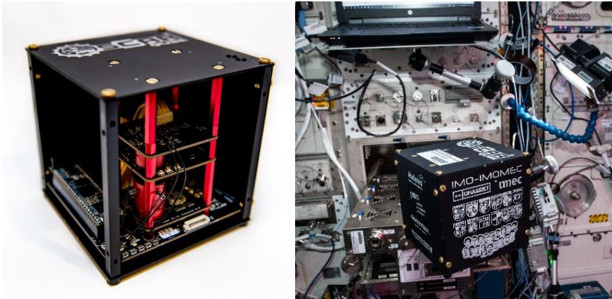
Fig. 43. Left) The completely assembled device without the side panels. Right) The OSCAR-QUBE is shown in microgravity onboard the ISS during installation by Thomas Pesquet (ESA).
