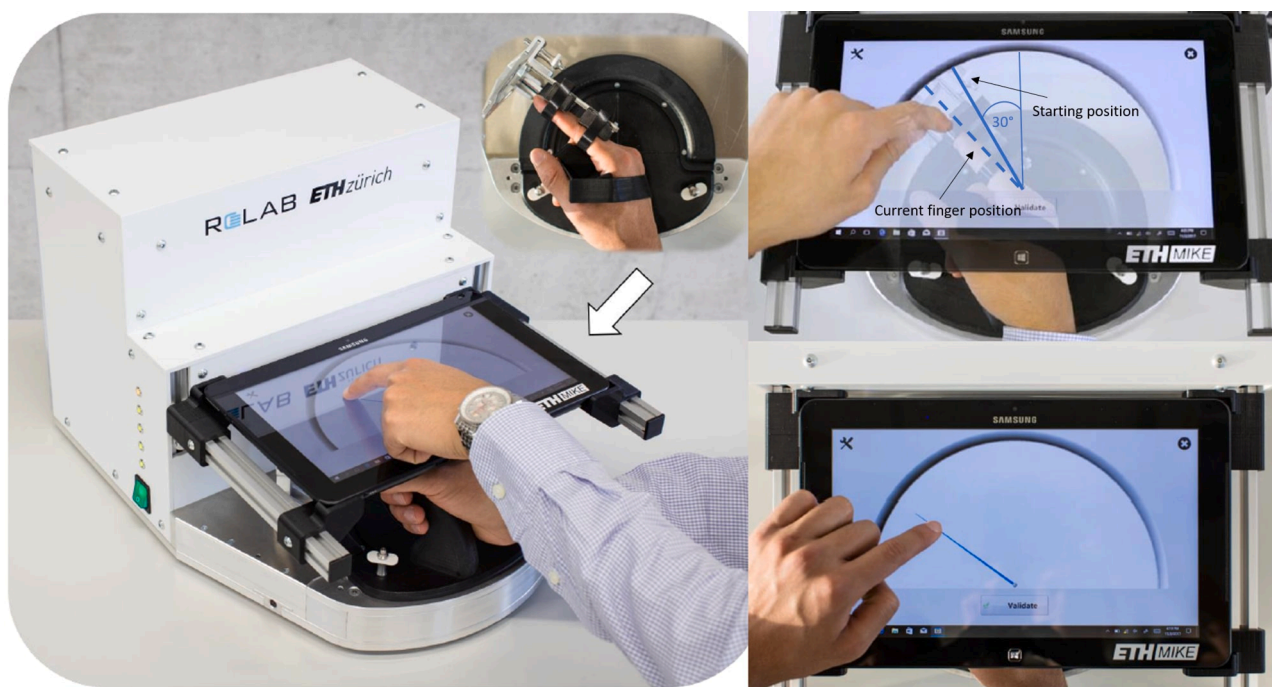
Fig. 1. The ETH MIKE device and its graphical user interface. This one degree of freedom end-effector robot can provide well-controlled displacement to the index finger, which is crucial for an objective and sensitive proprioception assessment. In the gauge position matching task protocol, the participant's finger is passively moved by the robot from a starting position ( 0^\circ angle at the MCP joint, 30^\circ from the middle of device's workspace) to another, random position. Then, the participant needs to indicate the perceived finger position on the tablet screen with a virtual gauge indicator, using the non-tested hand. When this was not possible because of impairments of the non-tested hand, the experimenter moved the indicator based on participant's oral feedback. This was repeated for 21 different positions (integer values [10-30^\circ] in flexion from the starting position).
