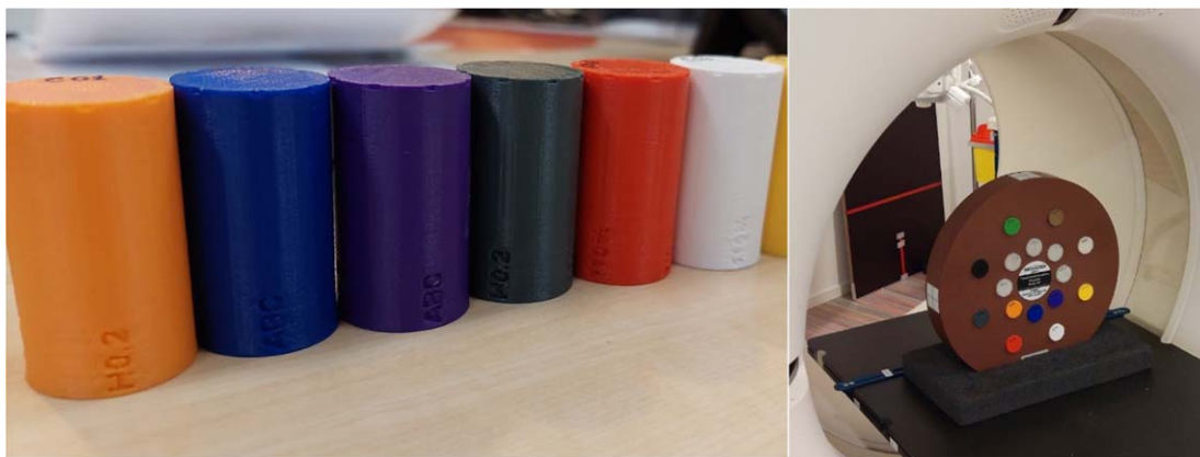
Figure 1. (a) 3D printed samples used to evaluate the different materials; (b) 3D printed samples inserted in the Gammex phantom (33 cm diameter) during a CT acquisition. Images were reconstructed with an iterative reconstruction kernel Qr40 resulting in a voxel size of 0.732 \times 0.732 (pixel spacing) \times 1 (thickness) \text{mm}^3 .
