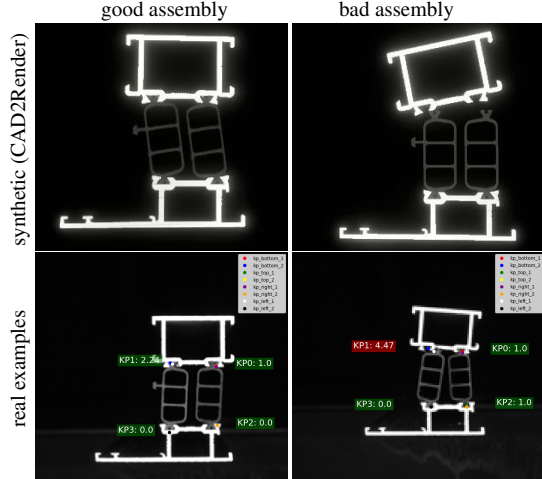
Figure 10. Assembly validation of good and bad assemblies. Top: synthetic examples generated with CAD2Render. Bottom: Output of the model shown on top of real examples in the case of a good validation (all points within spec) and a bad validation (one of the insertion areas show points that are too far from each other).
