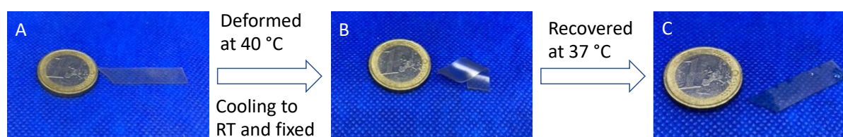
Figure 8. 4-PDLLA/PCL6-2K-AUP in its permanent shape (A) was heated, deformed and cooled down to fix the temporary shape. (B) Upon heating by immersing in a 37 °C water bath, the permanent shape is recovered (C).
