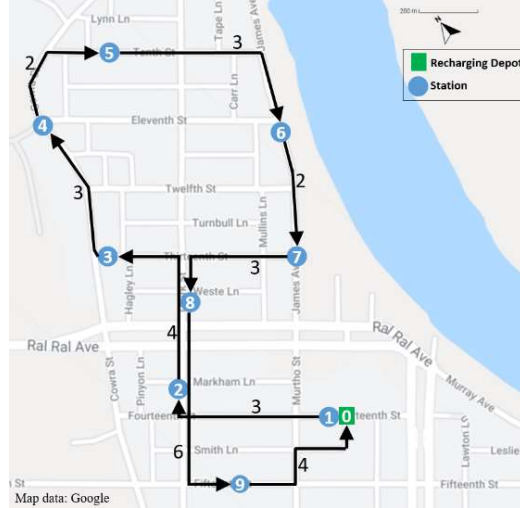
Figure 2: The eastern route of the driverless bus service in Renmark, Australia. Travel times in minutes are depicted on each link.
