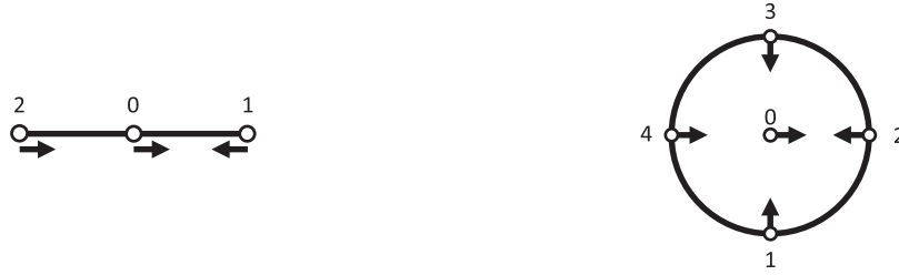
FIGURE 2. Numbering and directions of point forces in 1D and 2D. By considering the point forces with k \neq 0 and the limit |\mathbf{x}_0 - \mathbf{x}_k| \downarrow 0 , we obtain the point stress problem.
