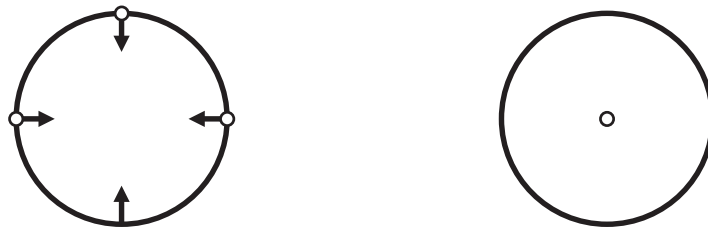
FIGURE 1. Left: contractive forces are defined on the cell boundary in the point force approach. Right: point stress approach employs an isotropic stress point source in the cell center.
