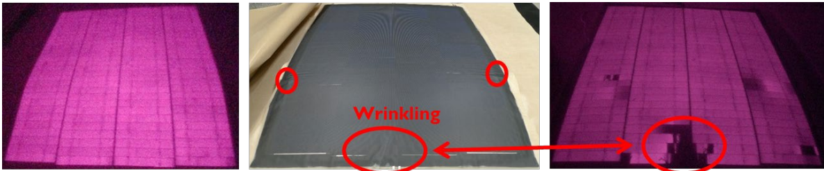
Figure 24: Severe wrinkling of the stiff back-and frontsheets induces cell cracks after lamination (central optical picture and right EL picture) in the shingled strings have no cracks whatsoever prior to lamination (left EL picture)
