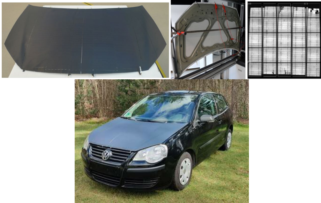
Figure 25: Fabricated full-size bonnet with a GFRB-based top surface and the original steel supporting structure: optical pictures of front (top left) and rear (top centre) and EL picture (top right), as well as a picture of the implementation on a car (bottom)
