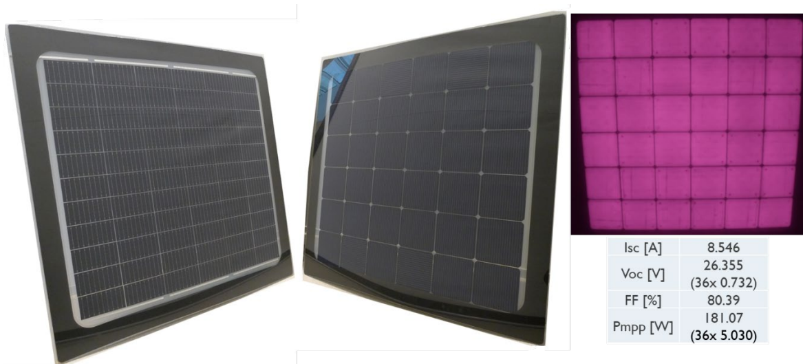
Figure 19: Optical comparison between sunroof with standard 9BB half-cell PERC strings (left) and 6x6 MW interconnected cells (centre), with EL picture and IV performance of the latter (right) (curved glass courtesy of AGP eGlass)
