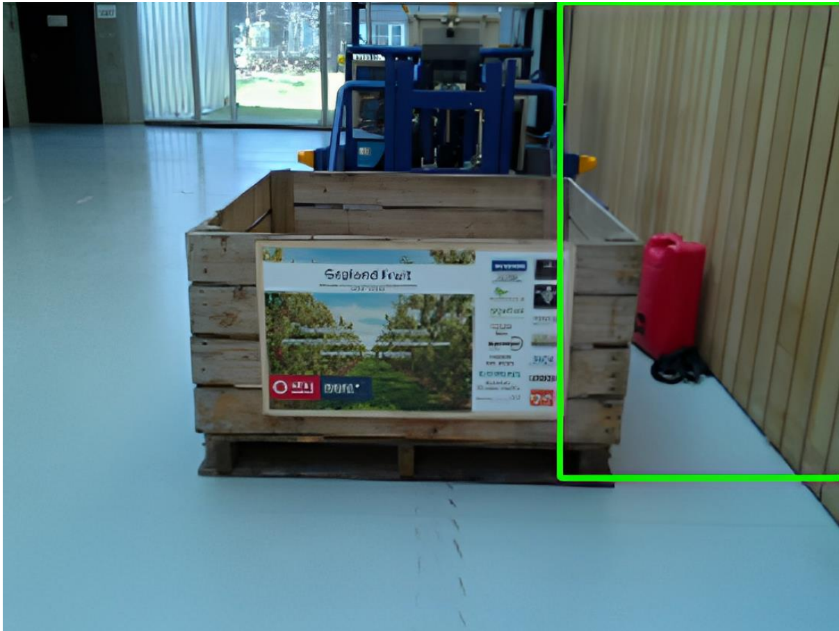
Figure 11: Failure case of using color-based filtering for bounding box extraction
