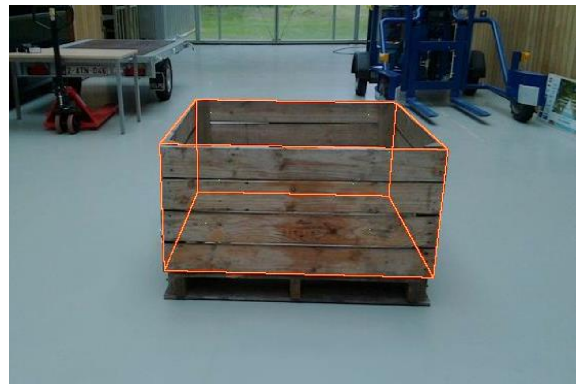
Figure 2: Visualization of the 6DPoseAnnotator program for obtaining the ground truth pose
