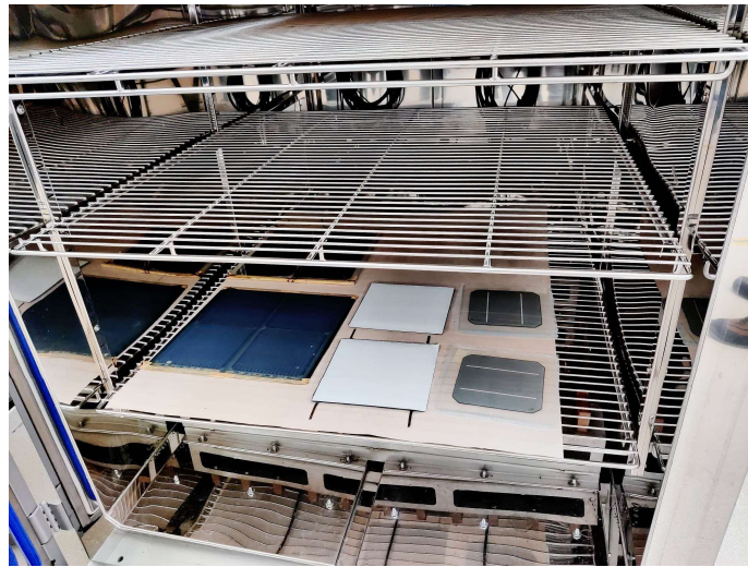
Figure 48: Damp heat chamber
