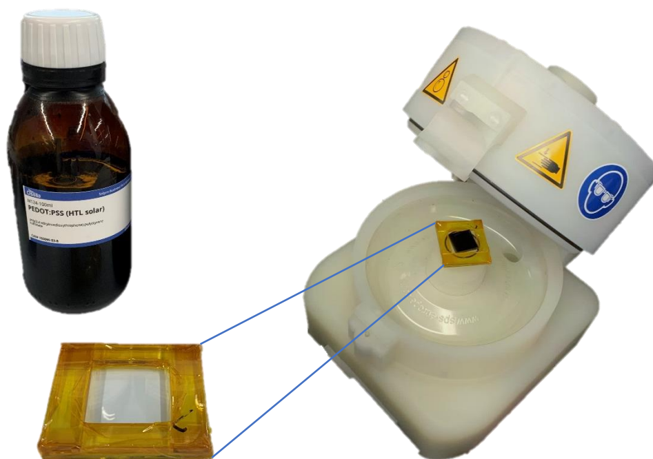
Figure 26: PEDOT solvent (top left), sample holder (middle) and spin coater (right).
