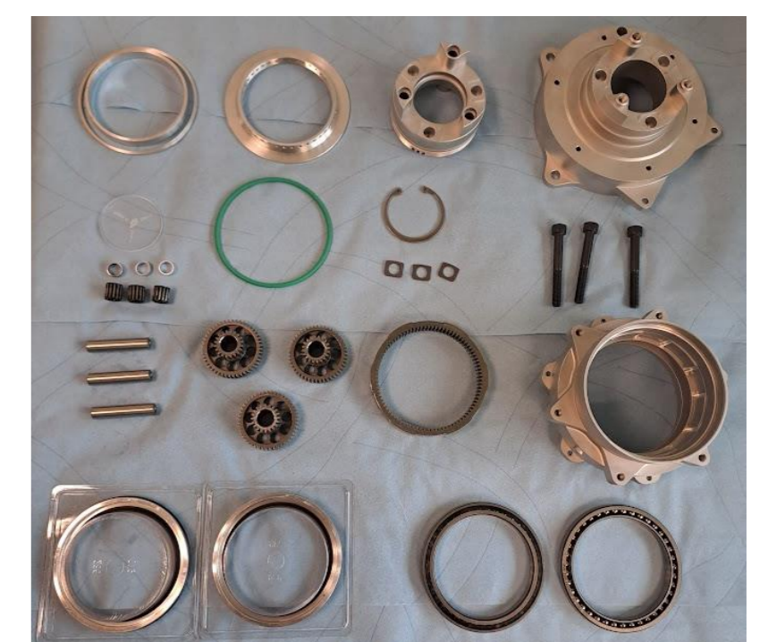
Fig. 7: Outrunner components lay-out
