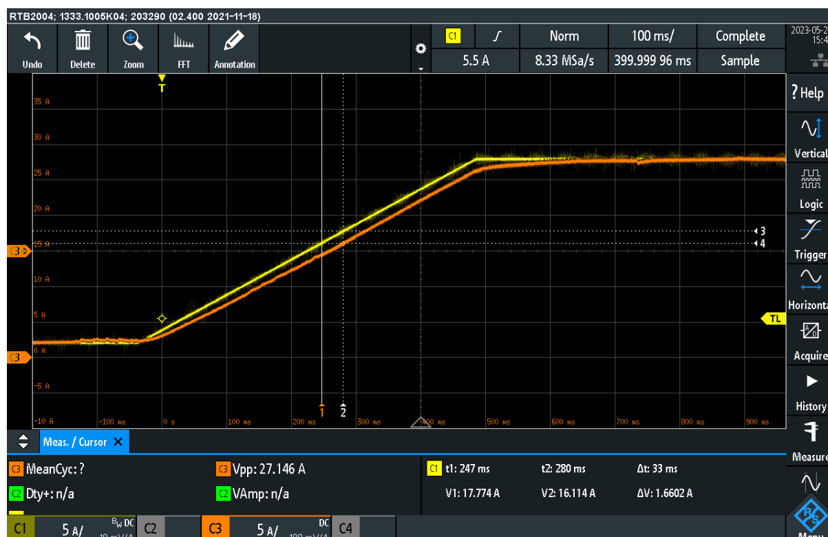
Figure 40: Oscilloscope screenshot during ramp response testing
