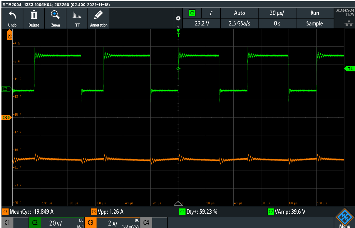
Figure 32: Oscilloscope screenshot during buck converter steady state operation
