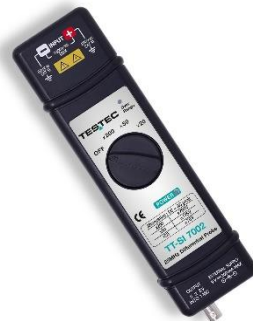
Figure 30: Example of a differential probe [22]
