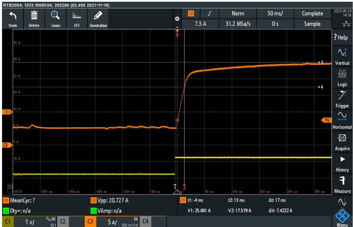
Figure 36: Oscilloscope screenshot during step response testing with the first control loop period
