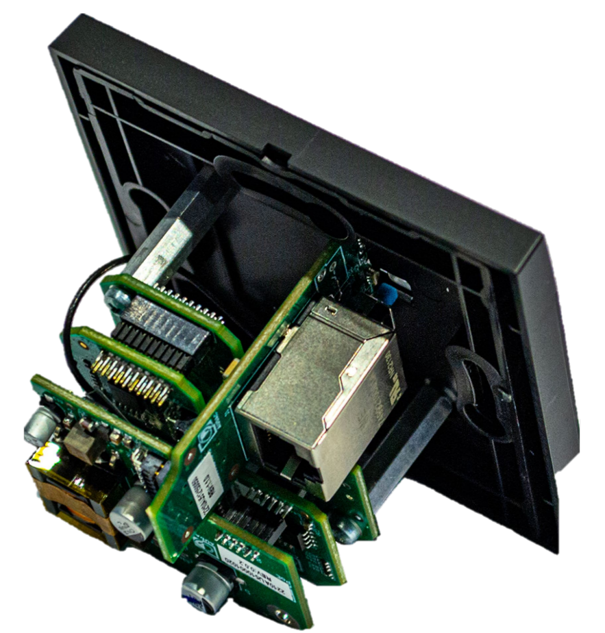
Figuur 2: Audac NWP400 USB/Bluetooth Wandmodule PCB-stack
