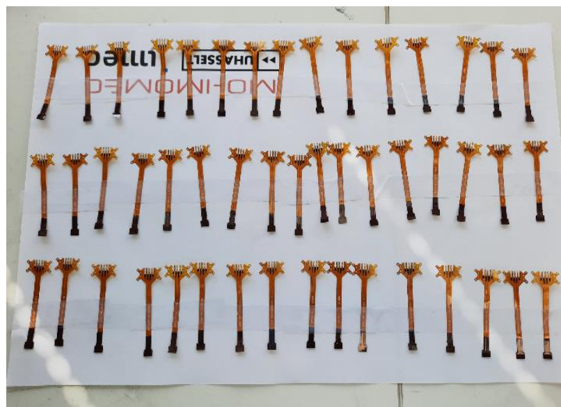
Figure 39: Flexconnectors positioned to apply primer
