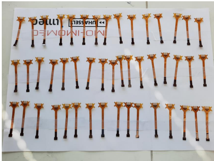
Figure A.7: flexconnectors positioned to apply primer
