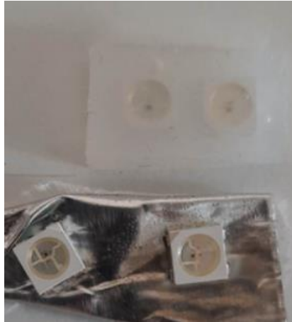
Figure 55: The four LEDs after three weeks of QUV testing
