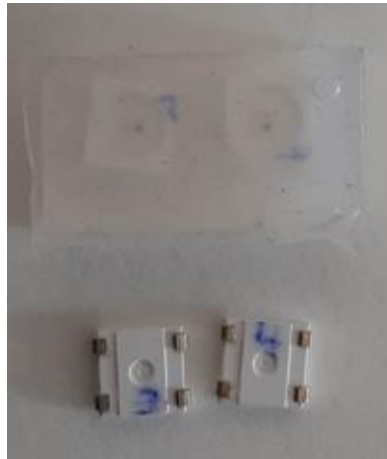
Figure 53: The four LEDs after three weeks of damp heat testing
