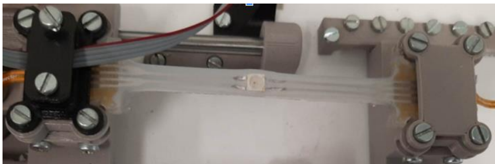
Figure 17: Ruptured prototype being stretched
