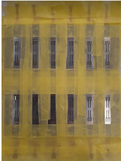
Figure A.13: stencil taped to the mold
