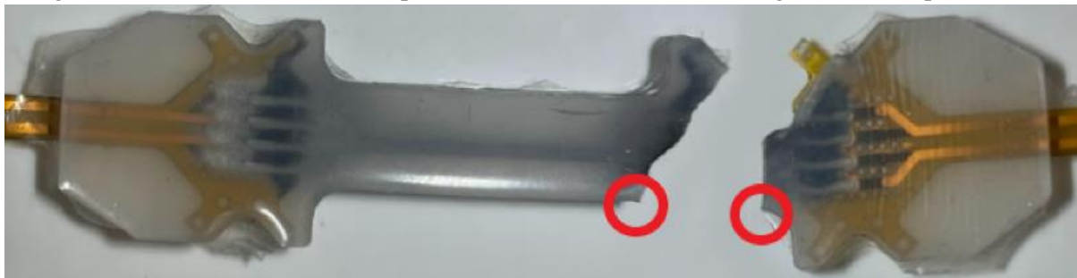
Figure 98: Batch 4 device 1, after rupture occurred at a weak point in the silicone device shape
