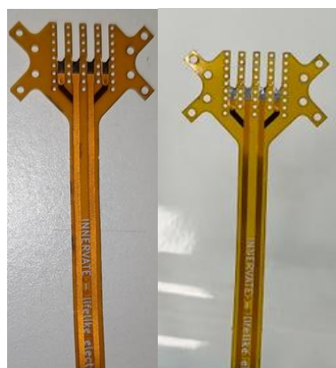
Figure A.6.a: flexconnector before the prewetting process, Figure A.6.b: flexconnector after the prewetting process
