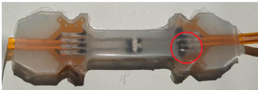
Figure 82: Two flexconnector legs sticking out of the silicone of device B2S2
