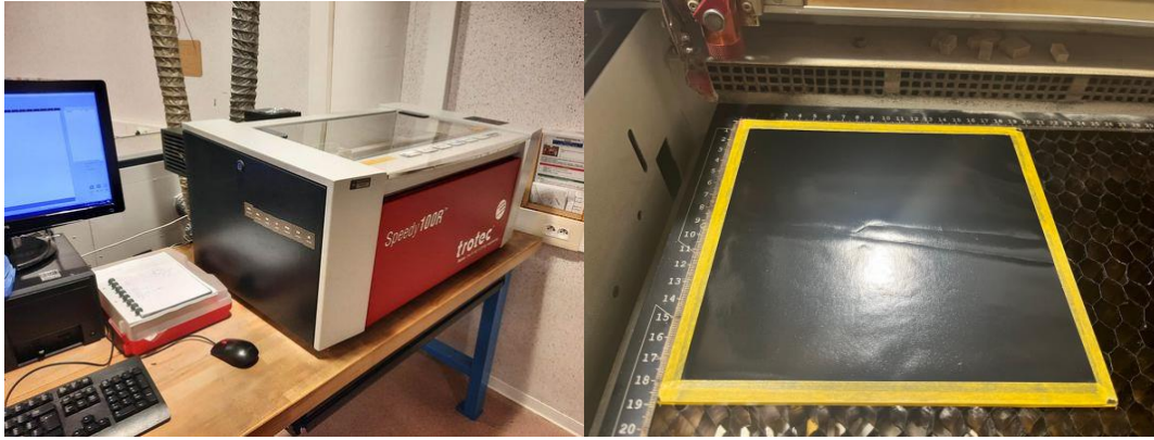
Figure A.3.a: Trotec speedy 100R, Figure A.3.b: base plate with vinyl in the laser cutter
