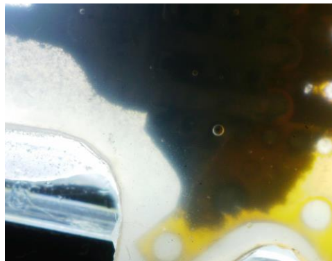
Figure 103: Batch 2 device 11, galistan migration to spacing between flexconnector and silicone
