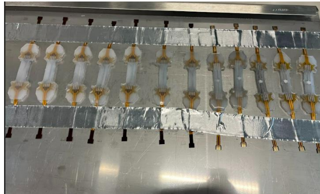
Figure 45: Devices as attached in the QUV chamber using metal tape
