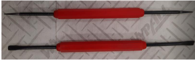
Figure A.17: tools that can be used to remove unwanted liquid metal
