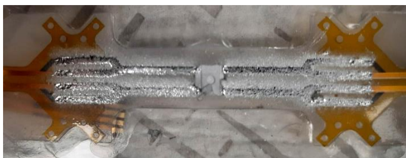
Figure A.16: possible short circuits between the traces
