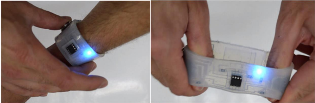
Figure 5: Stretchable wristband with sensors for input and output, power and processing embedded [8]
