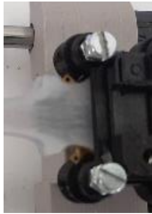
Figure 81: Front side legs of the flexconnector sticking out of the silicone of device B4S10
