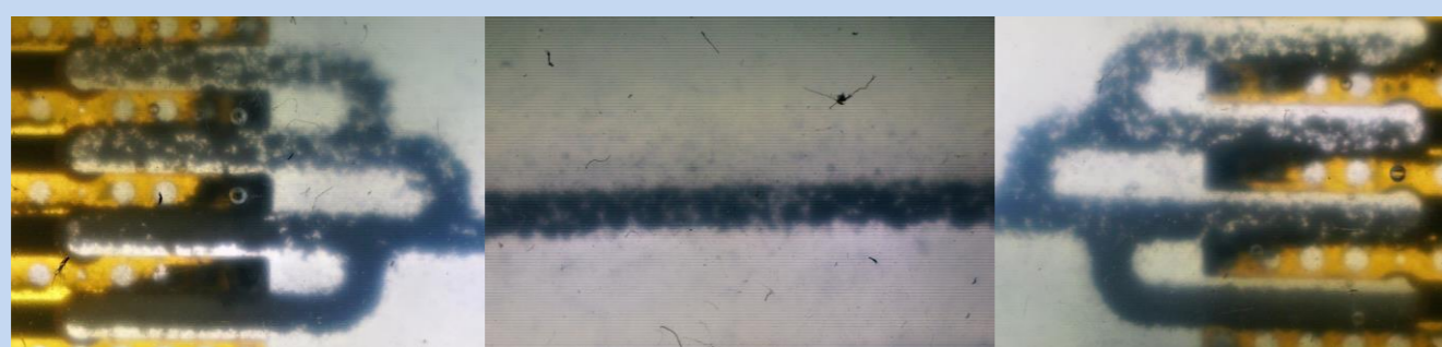
Figure 7: Close-ups of a stretchable wire after stretch testing
