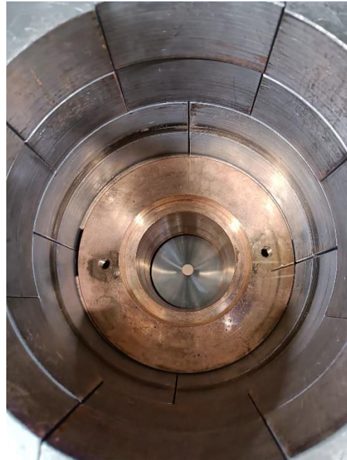
Figure 50: View inside the shield of the Ge-14 detector (the well is seen as the circle at the centre)
