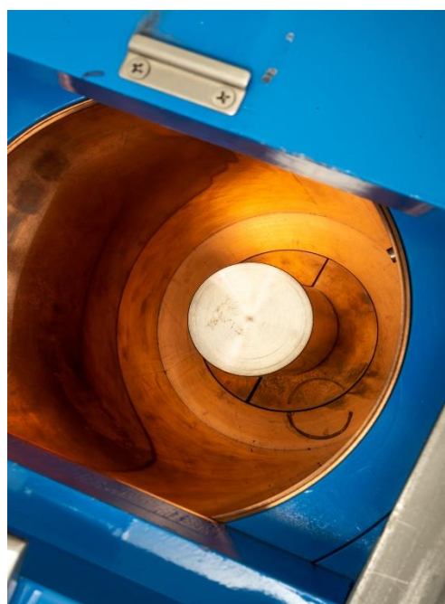
Figure 48: Look inside the shield of Ge-T10 detector
