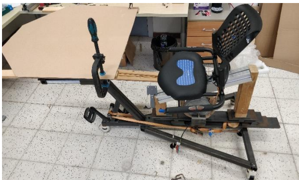
Figuur 17: Testopstelling geometrie cycling desk
