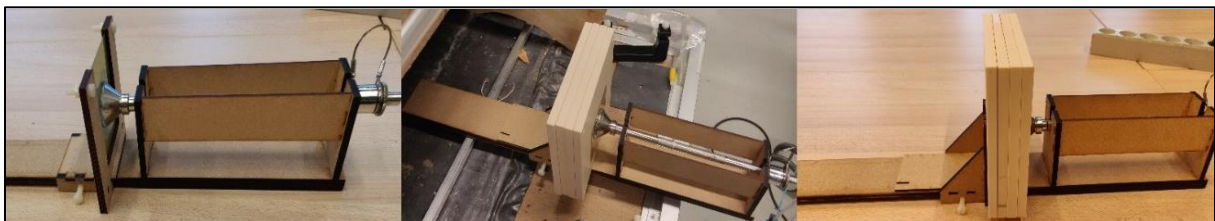
Figure 26: Experimental setups with measurements in air (left), on the surface of a 4 cm Plastic Water LR phantom (middle) and at 1 cm depth inside this phantom( right)
