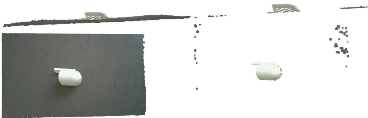
Figure 51: Original scene (left) and scene after plane segmentation (right)
