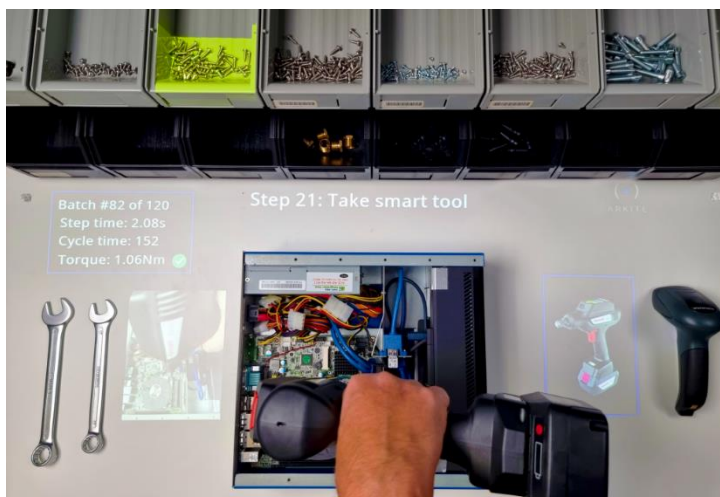
Figure 2: Projections provided by the HIM on the operator's workbench [5]
