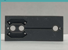
Figure 5: Top view fabricated LOC system
