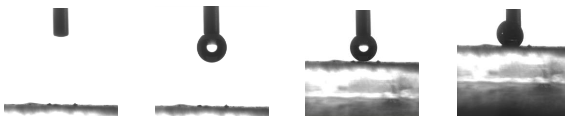
Figure 133: Traditional sessile drop technique
