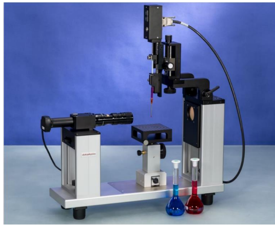
Figure 28: OCA 15 system from DataPhysics (USA) [84]
