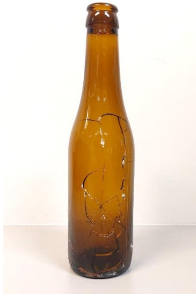
Figure 34: Fracture due to impact after freezing bottle A filled up to 10 cm
