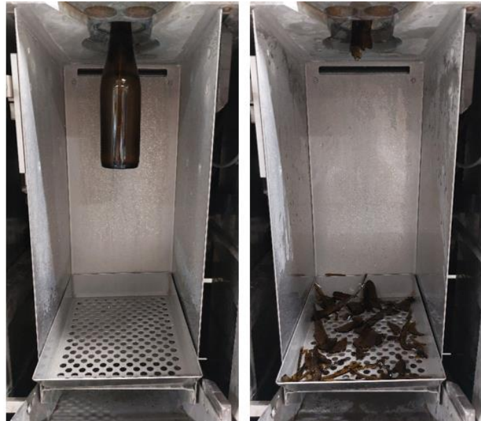
Figure 16: Bottle before (a) and after (b) breakage as a result of Destructive IPR test
