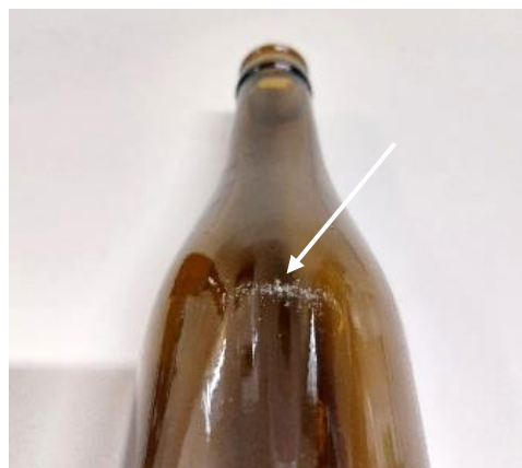
Figure 43: Scuffing after line simulation (5 min – 60 RPM – 40% slip)
