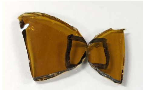
Figure 42: Fracture after IPR (26.3 bar) with fracture origin located at impact site
