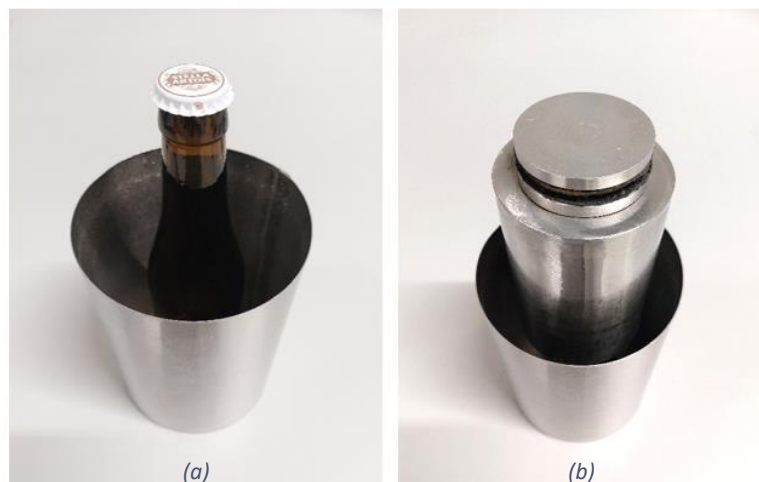
Figure 21: Bottle with crown cap inside cullet can without (a) and with (b) upper lid
