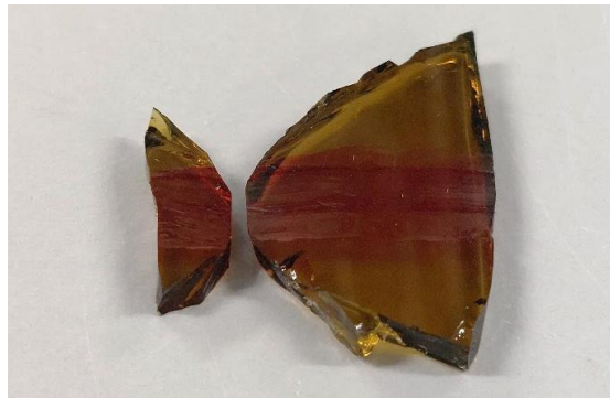
Figure 50: Fracture after IPR (30.5 bar) with fracture origin located at scuffing area after scuffing simulation
