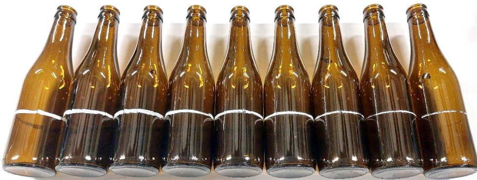
Figure 51: Visible scuffing after 10 minutes ranked from most to least severe
