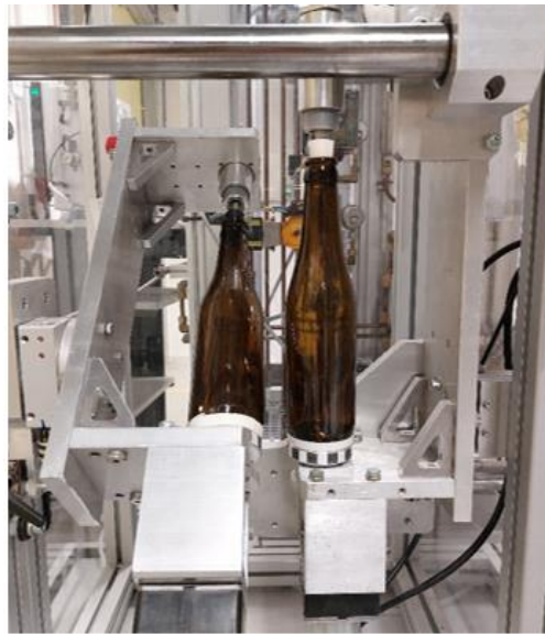
Figure 26: Angle of 45° between the bottles during scuffing simulation
