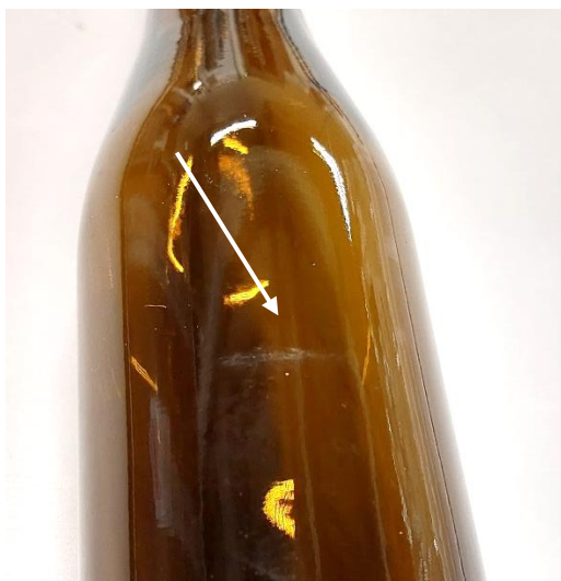
Figure 48: Slightly visible damage after scuffing simulation
