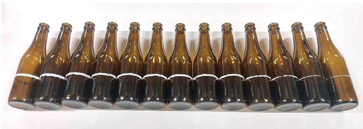
Figure 52: Visible scuffing after 15 minutes ranked from most to least severe
