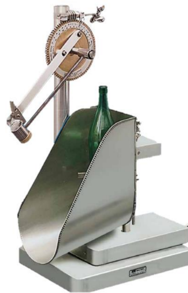
Figure 2: Pendulum striking a bottle at shoulder height [2]
