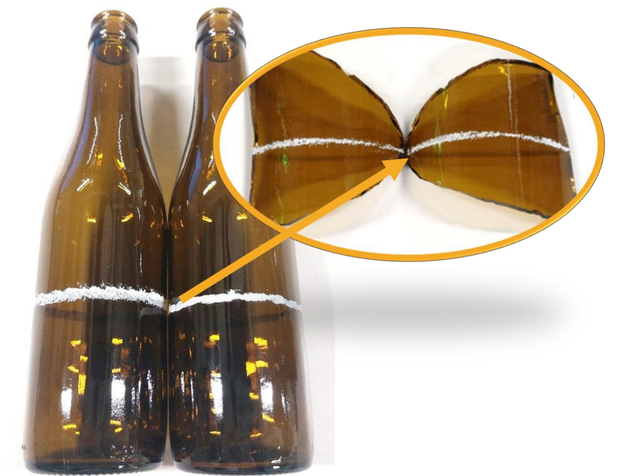
Figure 4: Pair of scuffed bottles with visual damage Detail : Fracture origin after friction was applied
