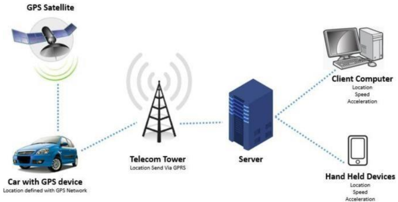
Figure 7: Naturalistic driving data flow process
