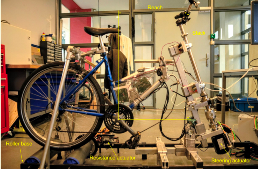
FIGURE 9 Construction of bicycle simulator (Dialynas, Happee, Schwab, 2019)
