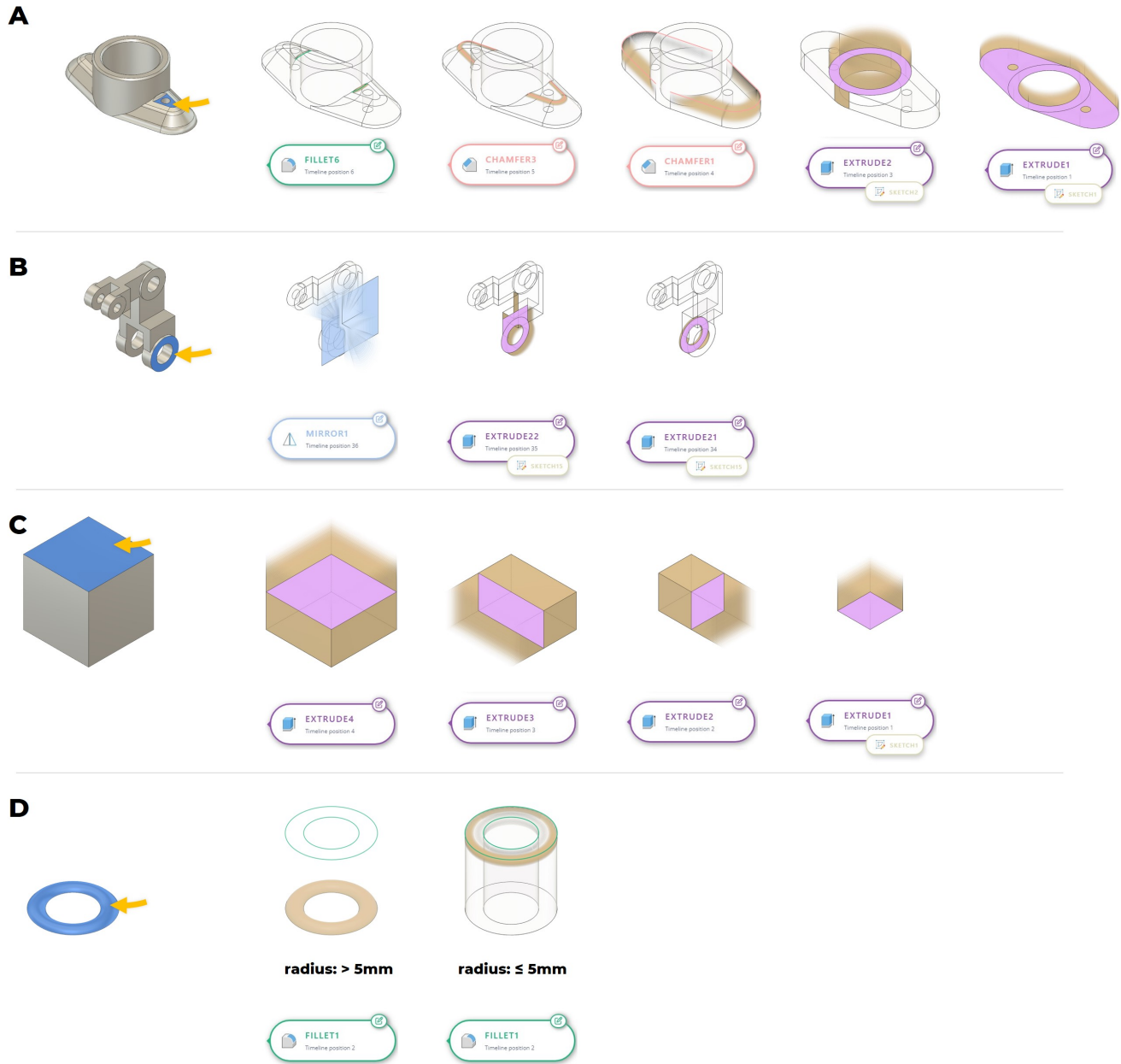
Figure 6: Some examples demonstrating the utility of HiM: (a) the dimensions of the selected face are not explicitly defined and are the result of several modeling features filtered and animated by HiM. (b) HiM informs the designer that the selected face is the result of a mirror feature. Changes to this face are thus also reflected in other faces. (c) HiM can help in understanding low-quality CAD models in which geometries are realized by duplicating modeling features instead of editing an existing feature. (d) The CAD model breaks when the radius parameter of two adjacent fillet features increases and the resulting curved edges start to overlap. HiM helps to recover such broken models.
