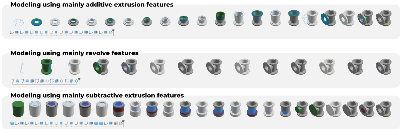
Figure 2: Three very different modeling histories in feature-based CAD modeling for realizing the exact same CAD model.
